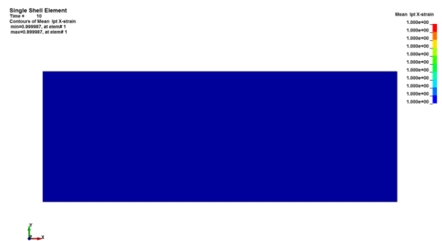
Fig. 3. True strain in the x-direction of the single element model. The final true strain is equal to 1 and the model matches theoretical value.
