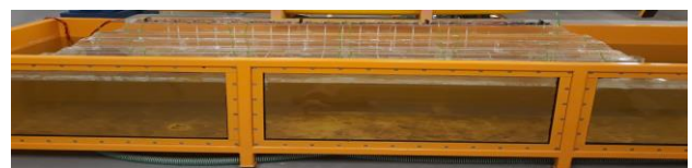
Fig. 1. The floating dock model scale 1:70 floating in the model basin
