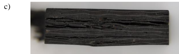
Fig. 1. Examples of photographs showing the laminate section after AWJ conducted with the following operating pressures: a) 1500 bar, b) 2500 bar c) 3500 bar
