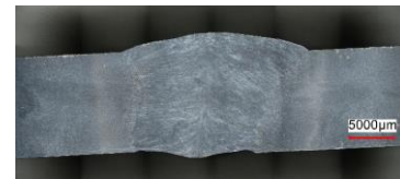
Fig. 2. Scheme of the butt welded joint of flat bars with welding groove
